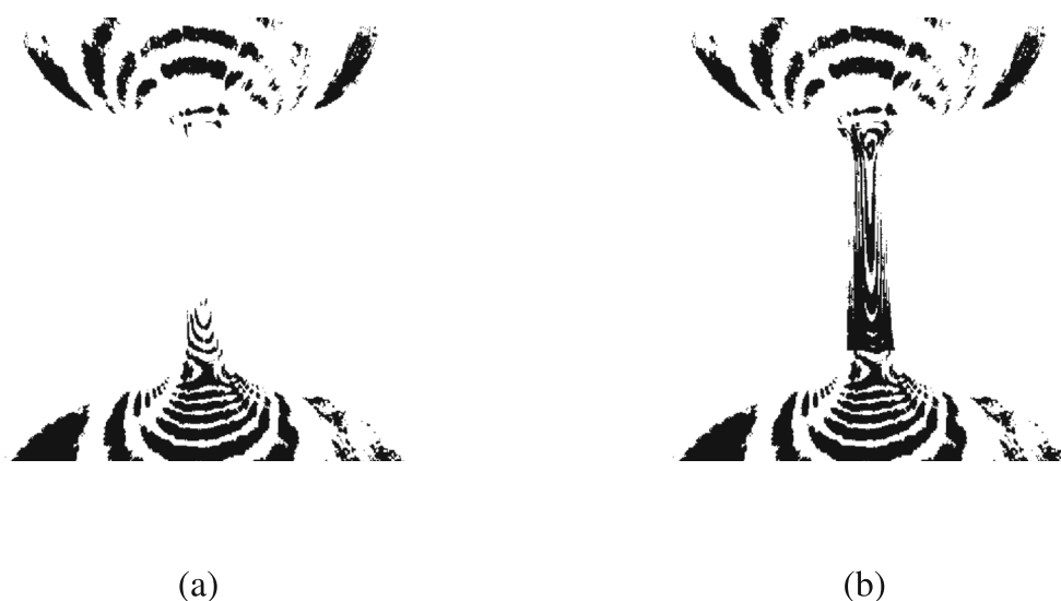
Fig. 27 Birefringence image binarization. a With a constant threshold. b With two levels of threshold
