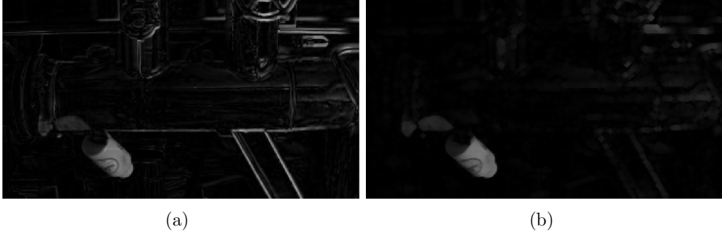
Figure 3.11: \mathbf{E}_e matrices before and after the application of the morphological opening. It is possible to note that the thin artifacts fade away while the object remains visible.
