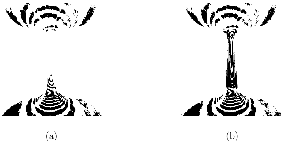
Figure 6.27: Birefringence image binarization. (a) With a constant threshold. (b) With two levels of threshold.
